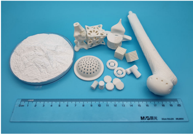
Fig. 1 Different 3D-printed calcium phosphate bioceramics. The customized 3D-printed calcium phosphate bioceramics can be used for maxillofacial bone repair, tumor bone defect filling, articular cup and elbow bone replacement
